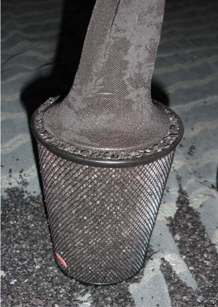
Now pull the end of the sock over the entire filter.. twist the end of the sock at the bottom and pull it up over the end of the cup.
